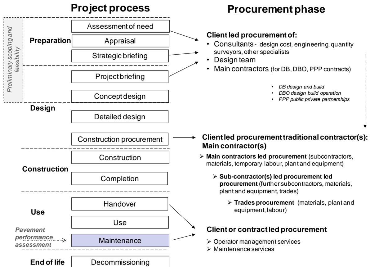
**Figure 1: Project process and procurement phases for road infrastructure (based on information provided in Berry and McCarthy (2011) Harmer et al., 2012, SUNRA project).**
